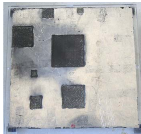
CDNE Corrosion sample with 0.040" deep corrosion pit of different sizes
